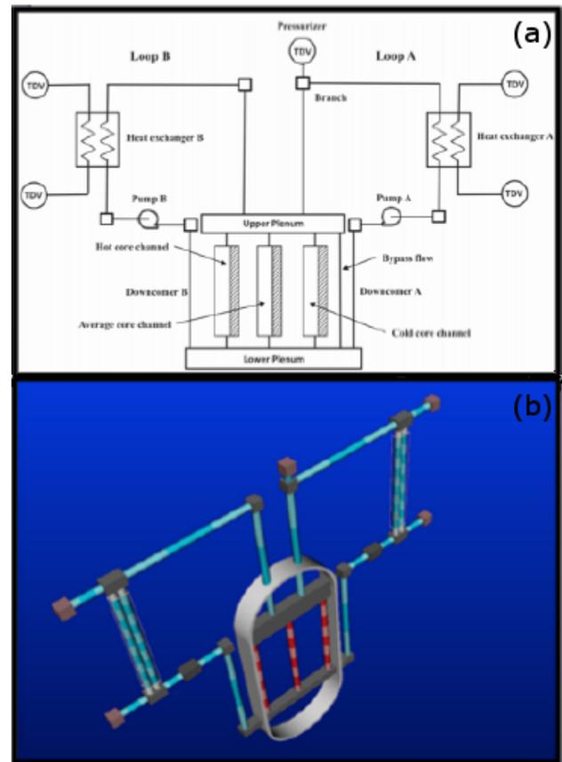
Fig. 1. PWR schematic (a) and RELAP-7 model (b)
