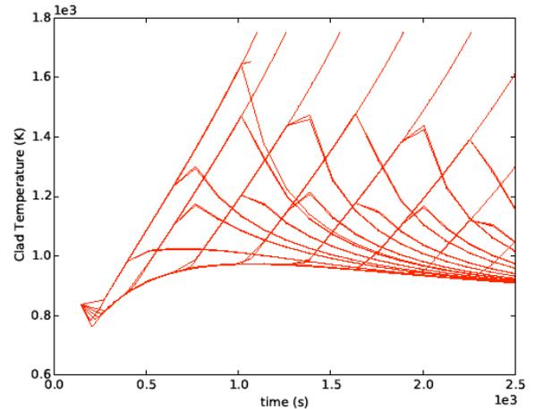
Fig. 2. Temperature of the cladding during grid sampled RELAP-7 runs
