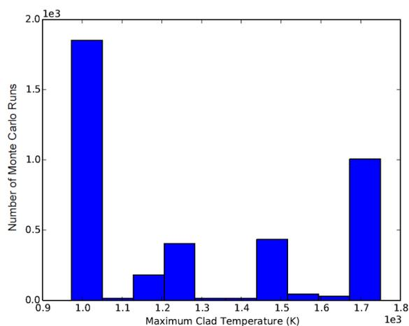
Fig. 3. Maximum temperature histogram of cladding during RELAP-7 (top) and surrogate model (bottom) runs
