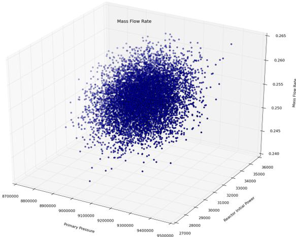
Fig. 1. RAVEN/RELAP-7 output: Mass flow rate response surface.
